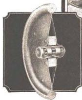
Sectional view of rubber tired disc wheel. (3 largest Auto-Wheels equipped with over-size tires.)
